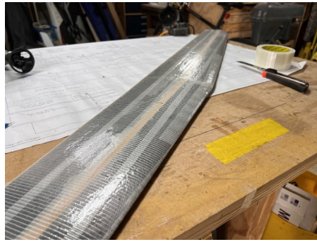
Cross weave tape, overlapped about 10mm
