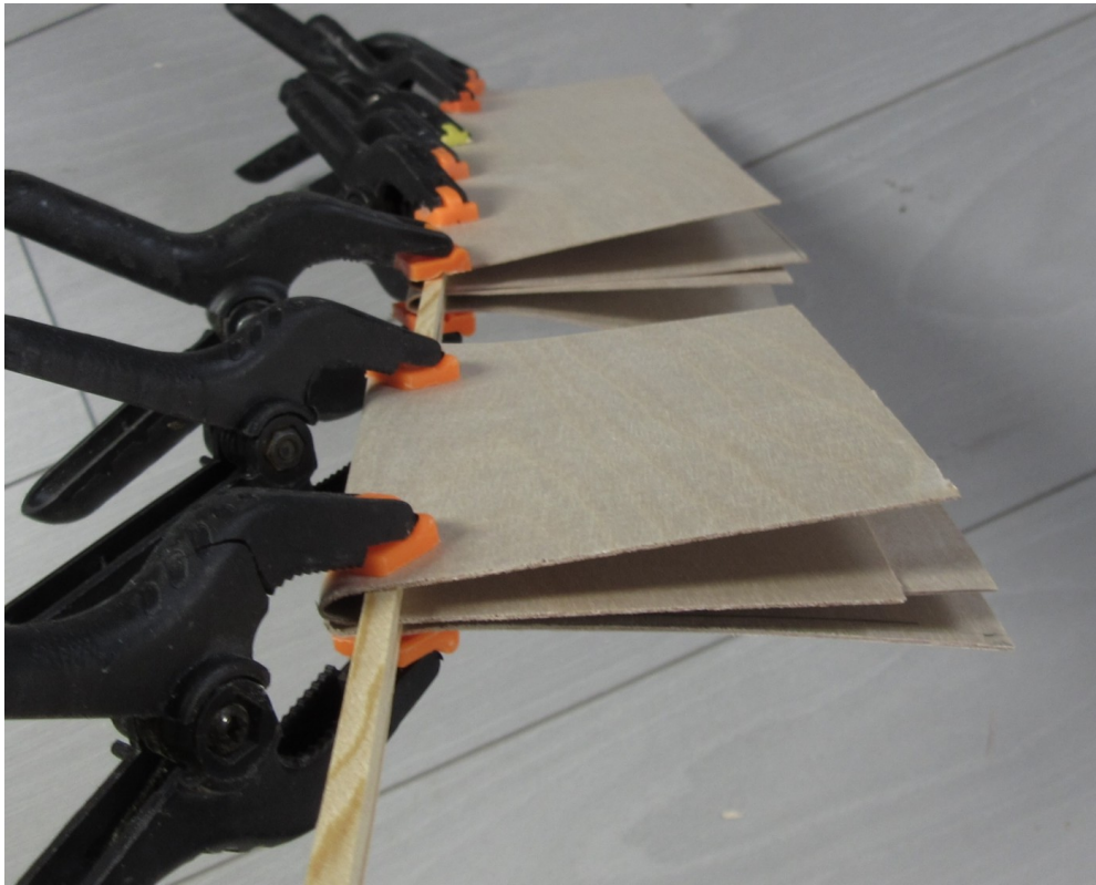
Wing sheeting ply pre-bent with boiling water.
