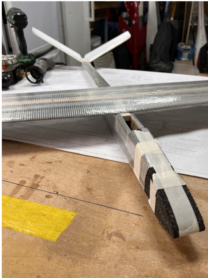
Control arms fitted and adjusted; equal throws confirmed. Time for a quick table fly.
