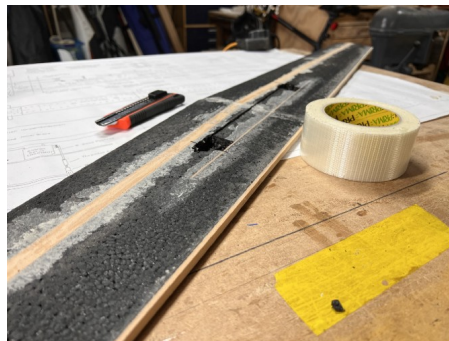
Mark the location of the servo pockets, rout them out with a Dremel and a jig.
