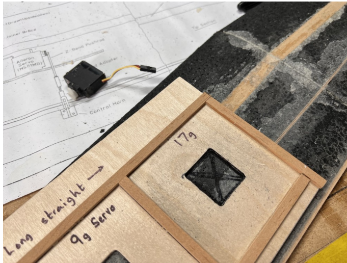
Mark the location of the servo pockets, rout them out with a Dremel and a jig.
