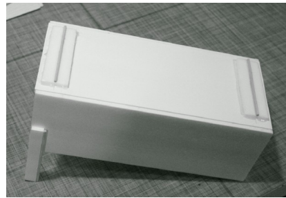
fig. 17 Dowel platform gully | fig. 18 Dowel hot glued into gully | fig. 19 Both dowels in place
