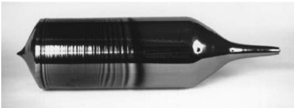
Picture 6: A silicon ingot. (credit: Solar Market Pty. Ltd.)
