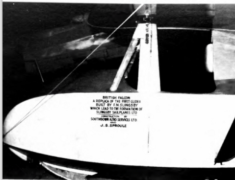
The replica Falcon, showing details of the cabane struts, skid and bracing wire. (M. Simons)
