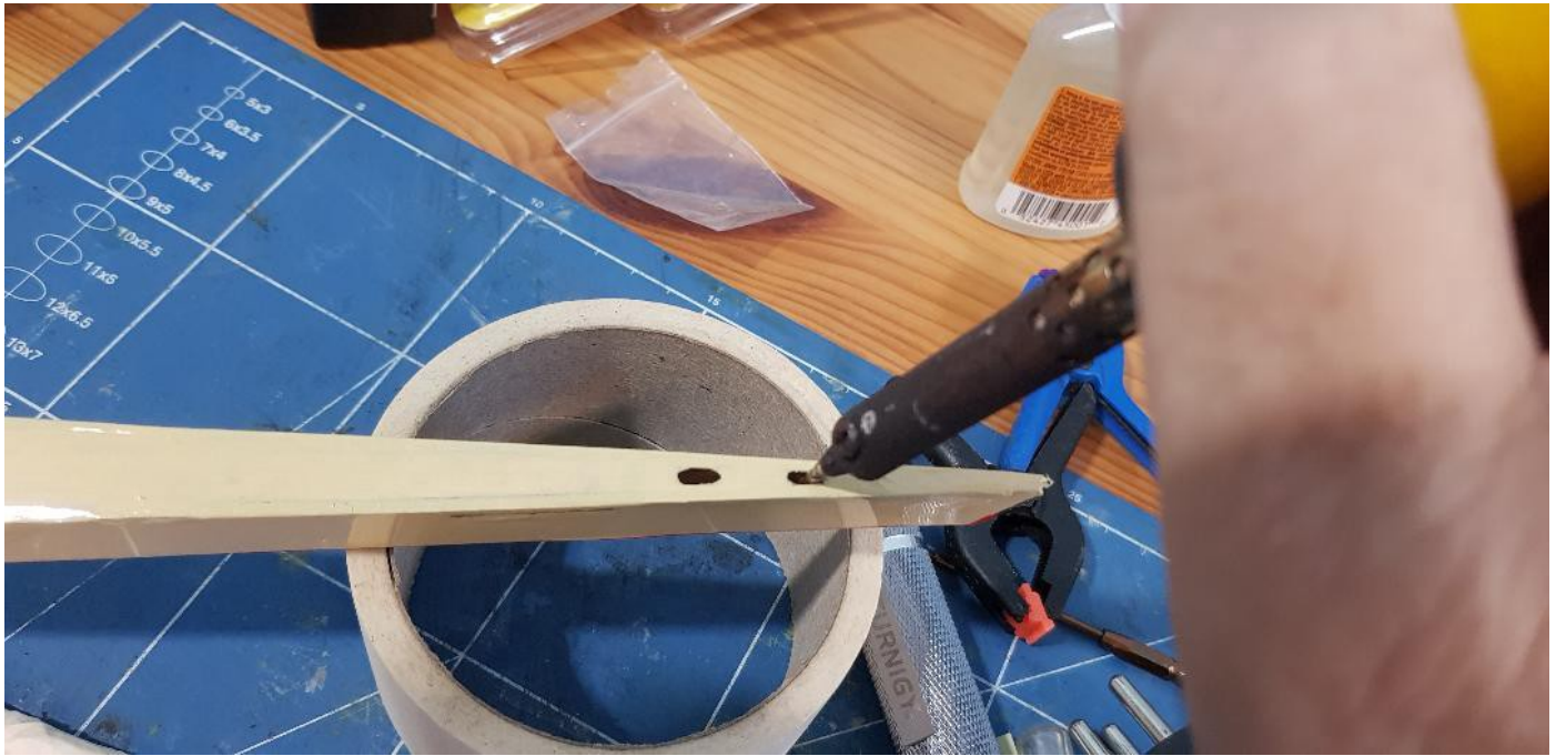
30: Opening up holes with a warm soldering iron.
