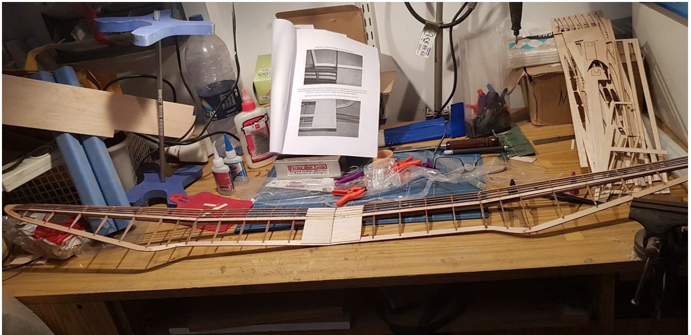
24: The completed wing, ready for covering.
