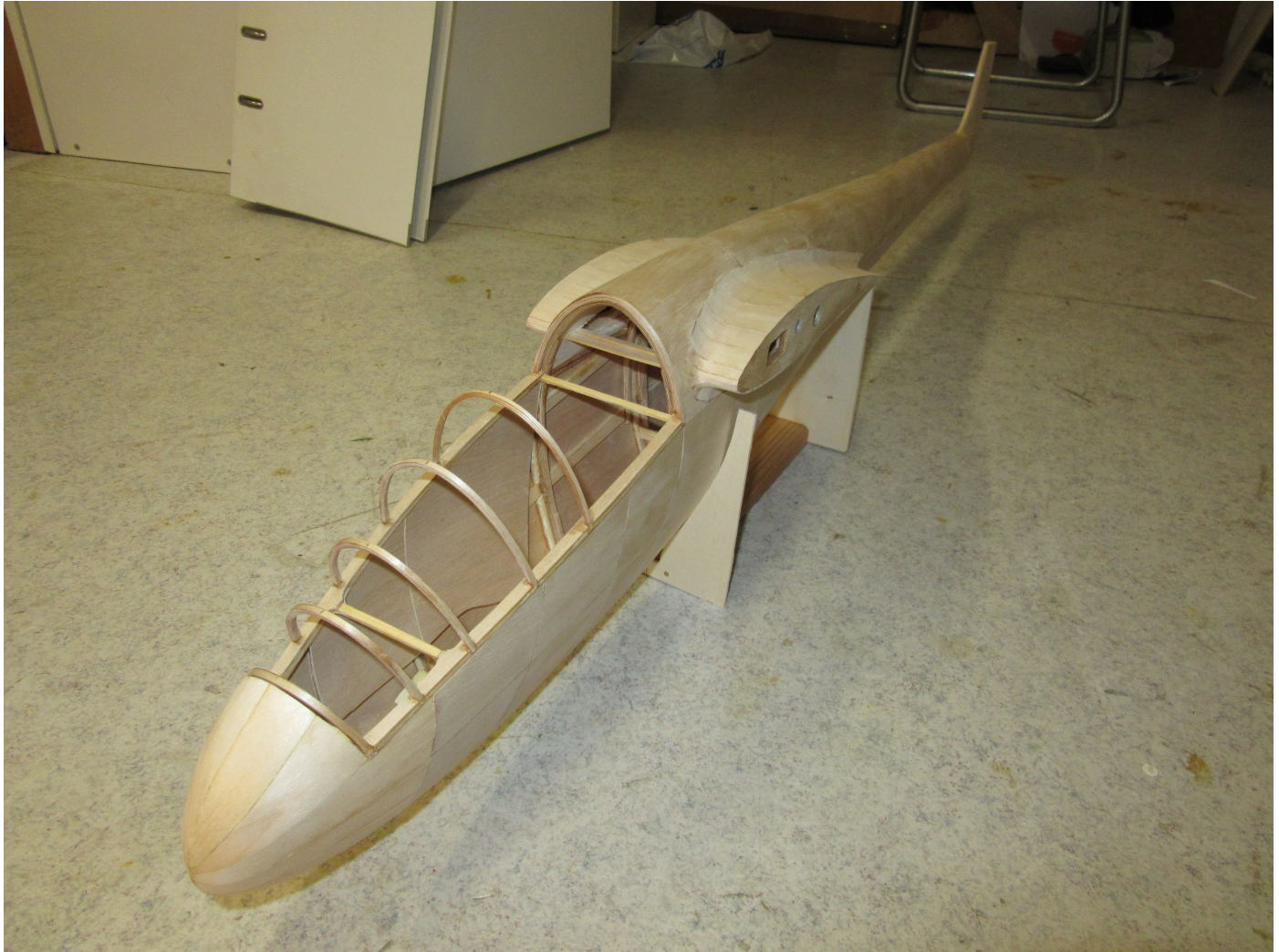
17 (top left), 18 (top centre): Bending ply across the grain. | 19 (top right): Glued in place. | 20 (bottom left): Fairing completed. | 21 (bottom right): Fuselage roughly finished.
