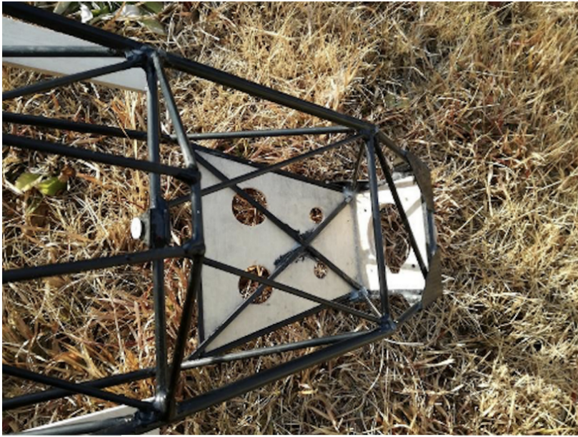
Photo 126: Back side of the motor mount.
