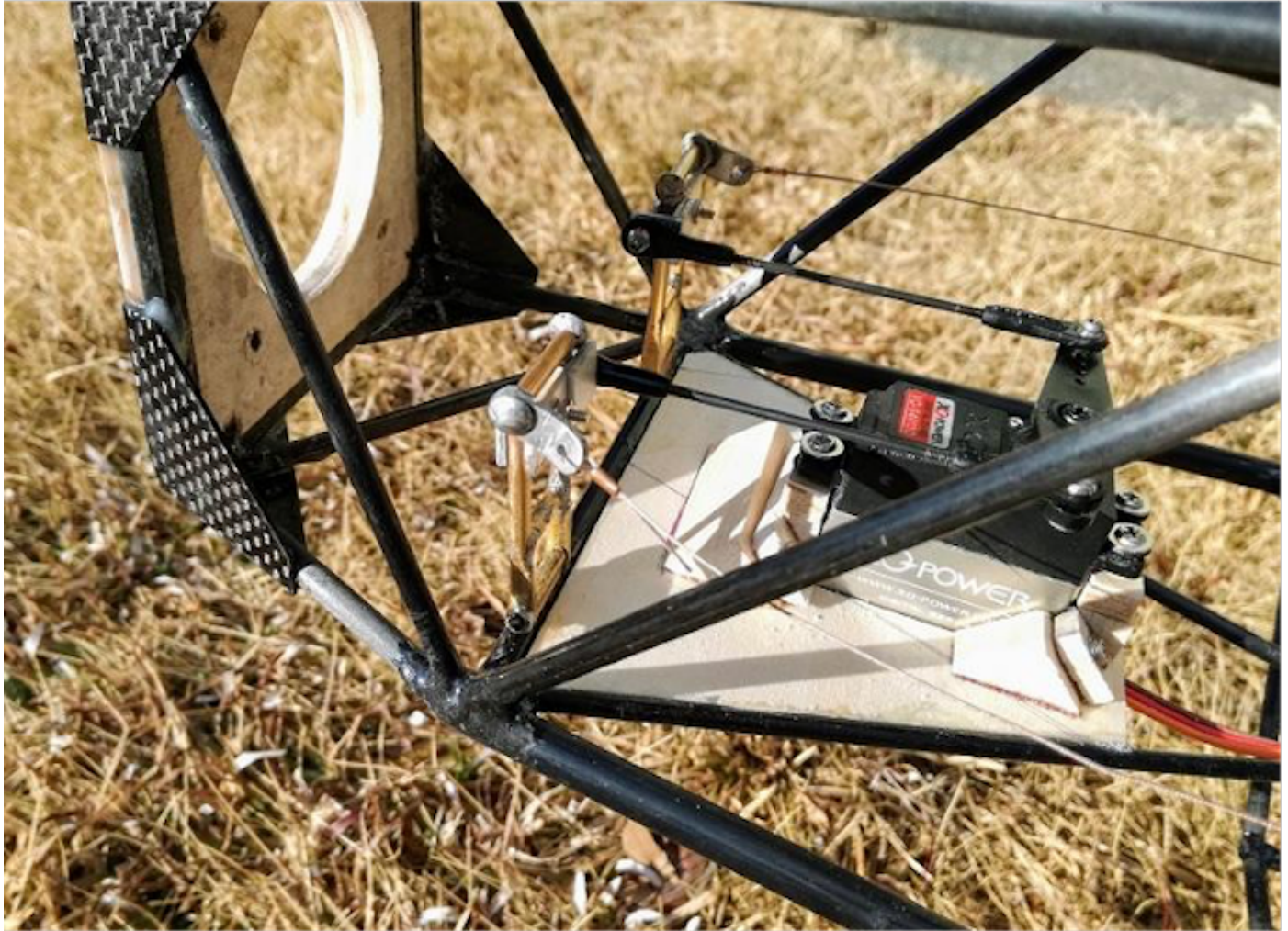
Photo 132: Installation of the rudder servo.
