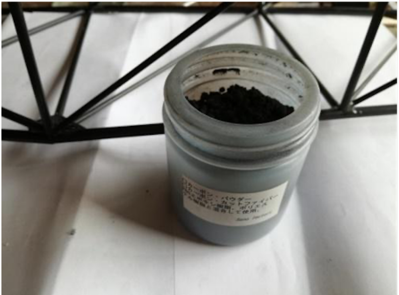
Photo 123: Carbon powder mixed with epoxy adhesive for bonding carbon truss structure.
