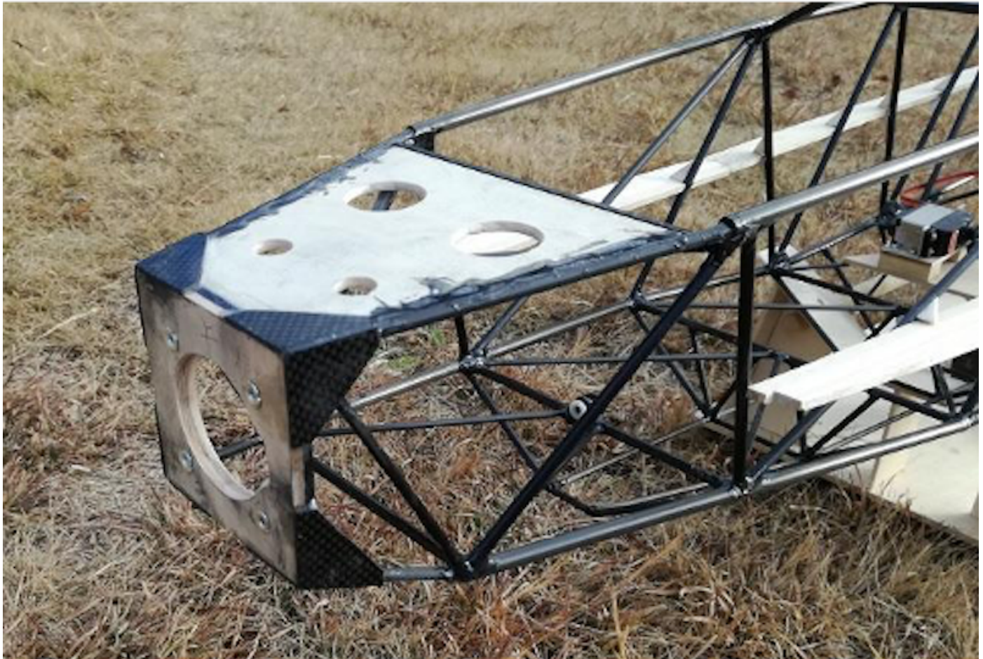
Photo 125: The completed motor mount.
