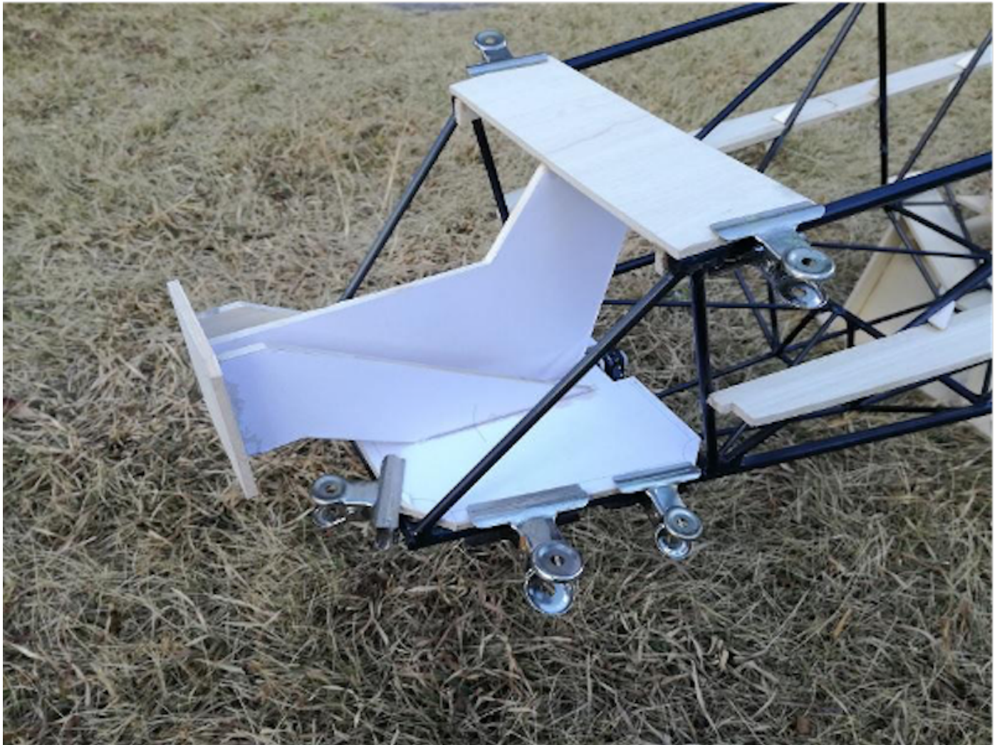
Photo 122: Motor mount assembly jig.
