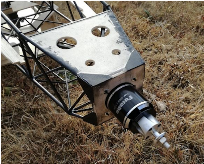
Photo 127: Temporary attachment of the motor to the mount.
