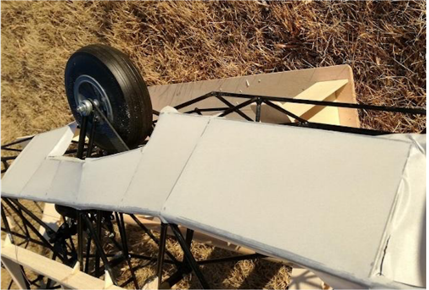
Photo 134 (left): Structure around the main landing gear seen from the front. | Photo 135 (right): Trial application of the Oratex.
