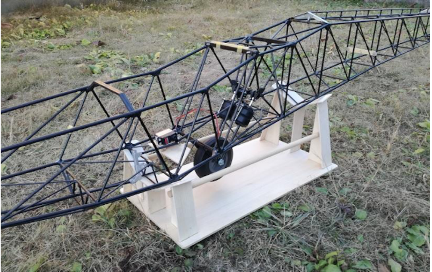
Photo 118: The completed fuselage rack.
