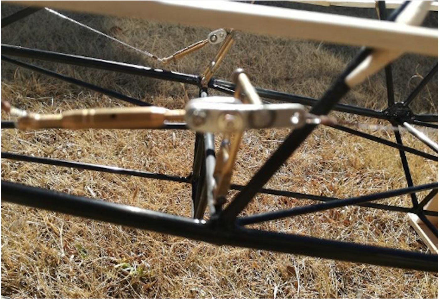
Photo 130: Installation of pedals Left, front seats. Right, rear seats.
