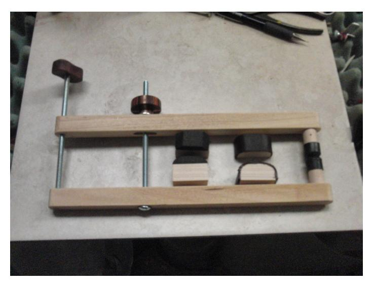
A simple flat clamp came in handy for gluing puzzle blocks and strips together.
