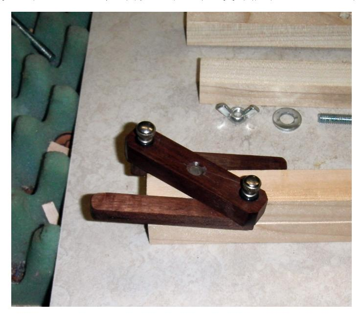
Stack the two pieces and drill a 7/32" hole through the top piece and deep enough to mark the bottom piece. Remove the top piece and drill the bottom piece half way through with a 9/32" bit. Thread the top piece with 1/4–20 tap. You can use the bolts if you don't have a tap. Harden the wood threads with CA. If you only have soft wood, you can use 1/4 -20 threaded inserts, but I did not find it necessary with the wood I had.
