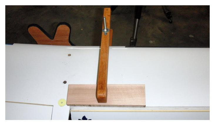
The Long Reach Clamp works great on a trailing edge spar, for example.
