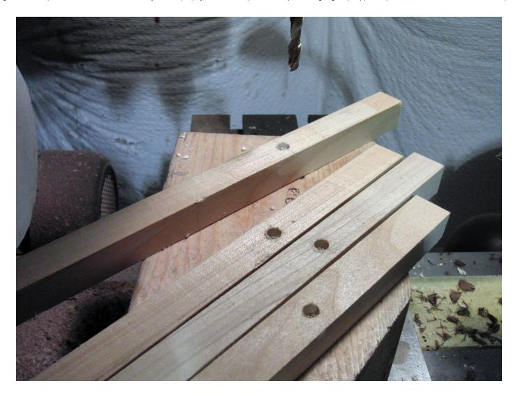
Mark for the slot — 3/4" to 1" wide. This helps keep the screw from jamming when at different angles during clamping. Drill a 5/16" hole at each end of the slot. Drill out the stuff in between. It is cleaner if you use a knife and score down the sides between the holes.
