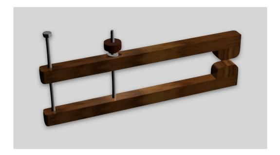
So...I came up with this very simple, easy to make clamp. A bit more versatile than the standard wood or fiddle clamp. The size can vary depending on how you want to use the clamp. I made 12" clamps because that was the material length I already had left over from making a bunch of wooden puzzles and it would suit my purpose.
