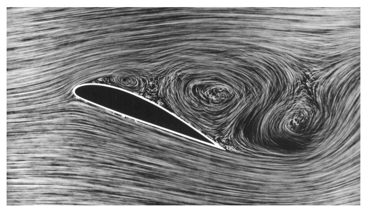
Photograph of an airfoil in a wind tunnel showing separated flow over the top surface, taken in 1915. (image: Deutsches Zentrum für Luft- und Raumfahrt via Wikimedia under Creative Commons Attribution 3.0 Germany [CC BY 3.0])
