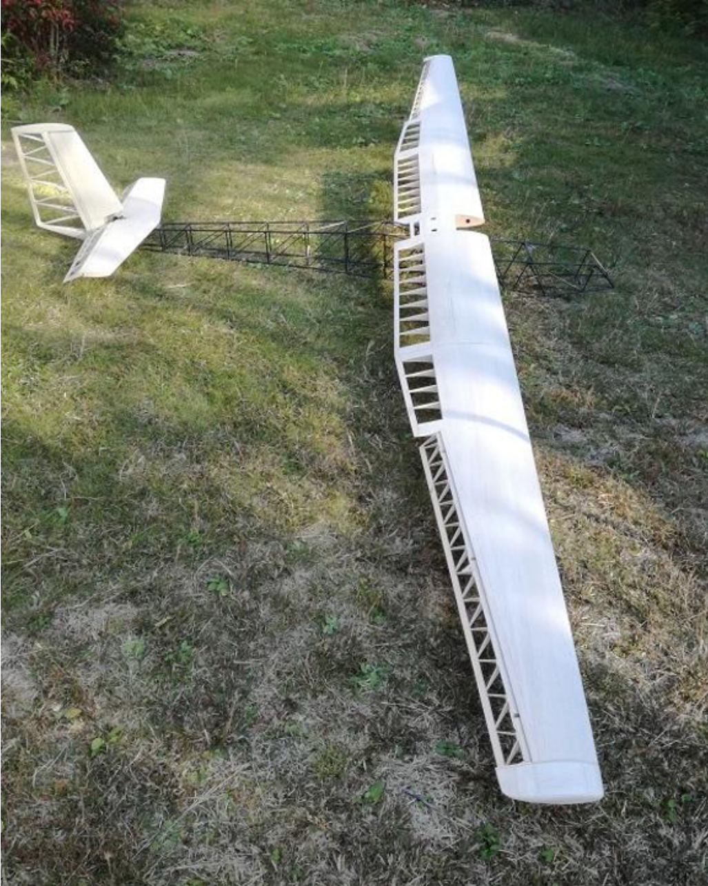
Photo 110: Main and tail wings assembled on the fuselage.
