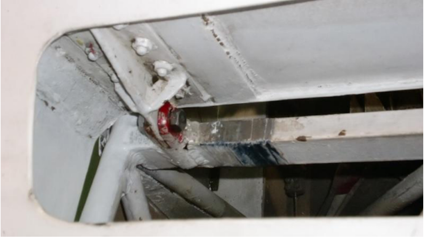
Photo 95: Fittings of rear spar and fuselage of actual model.
