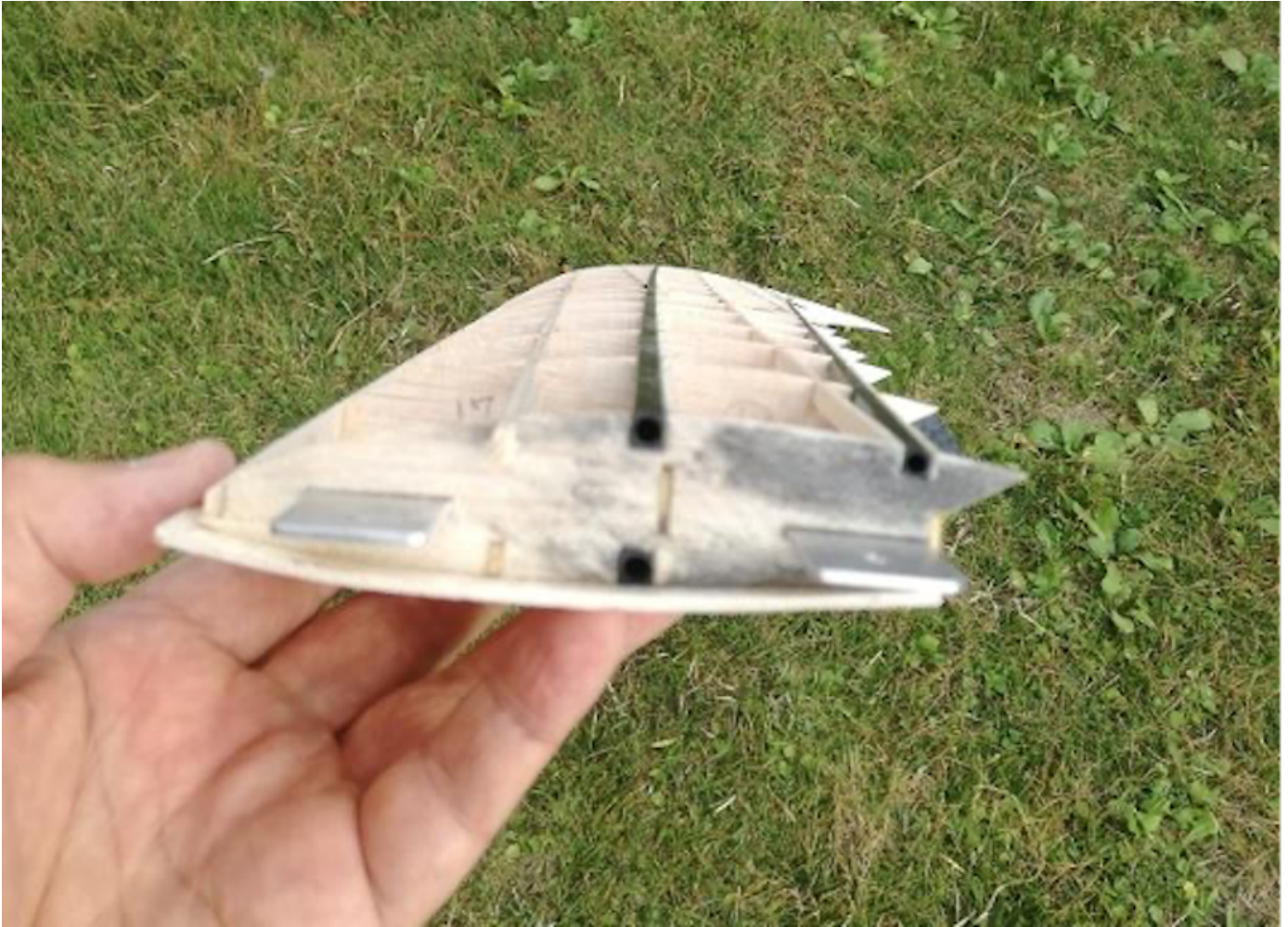
Image 103: Deformation of the outer wing spar.
