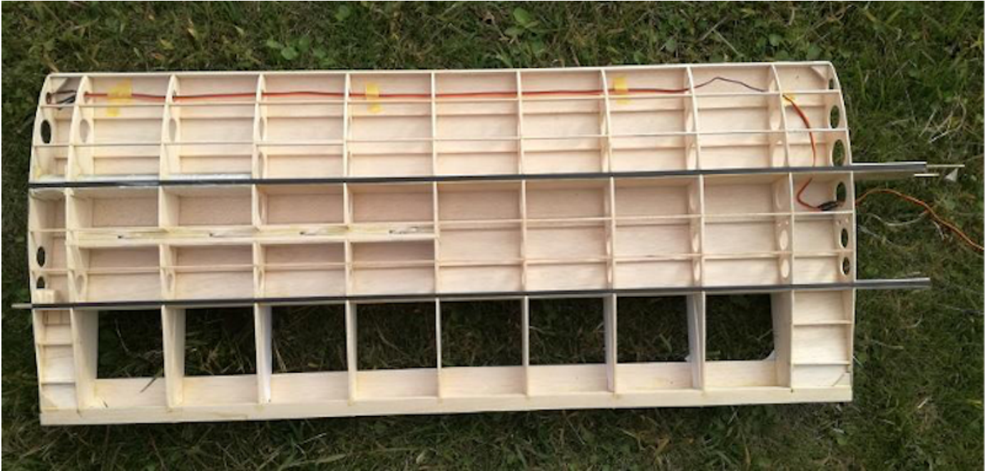
Photo 92: Left side center wing with the lower plank completed.
