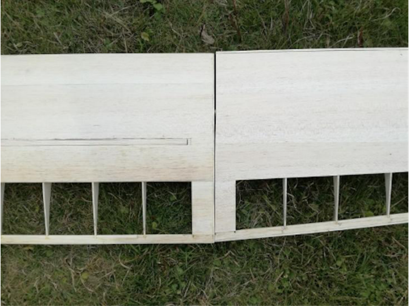
Photo 107: The connecting surfaces of the center wing and the outer wing do not meet!
