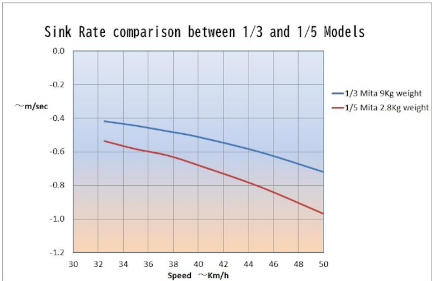
Graph 13: Comparison of the sink rate between 1/3 and 1/5.
