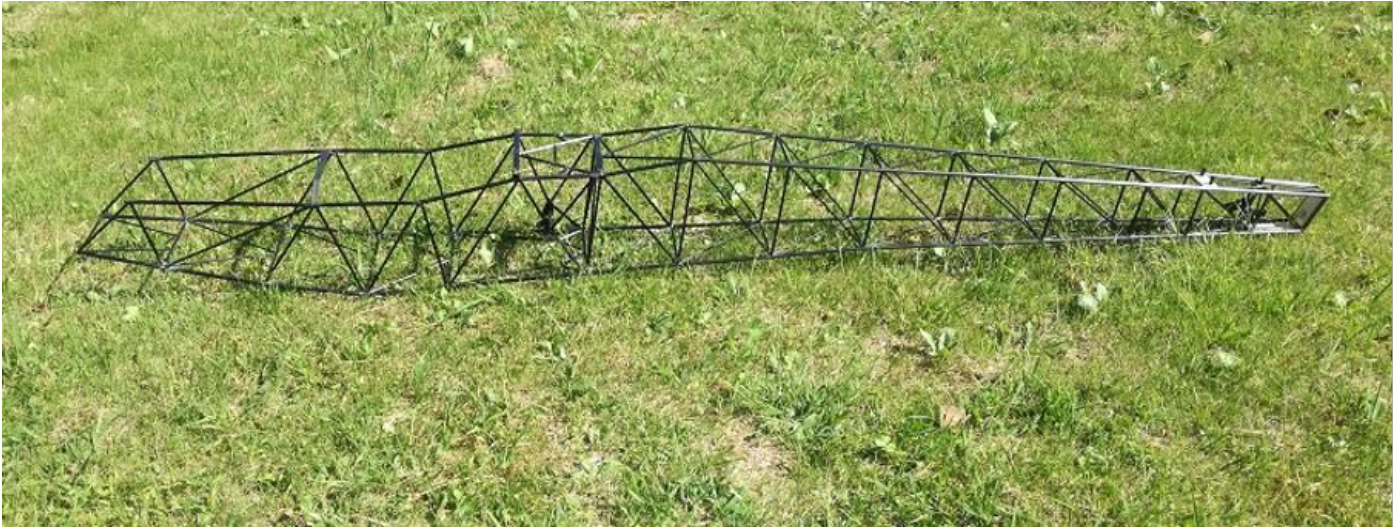
Photo 77: Main structure of the completed fuselage.
