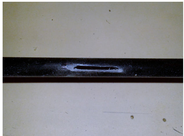
Photos 10 and 11: I cut a slot in each side of the tube about 3/4 in long.
