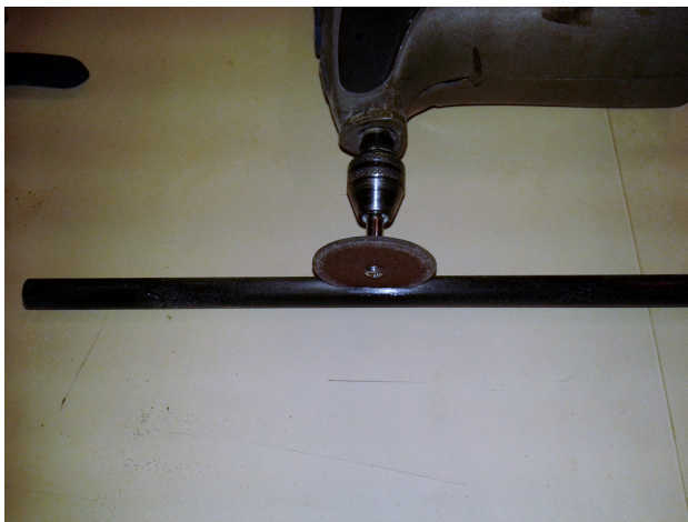
Photos 10 and 11: I cut a slot in each side of the tube about 3/4 in long.
