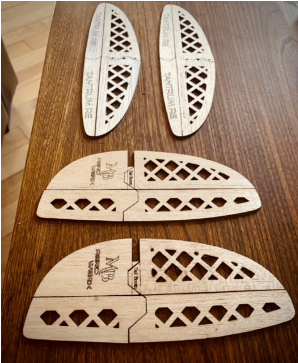
Photo 8: Laser cut tail feathers with some cool looking lightening holes.
