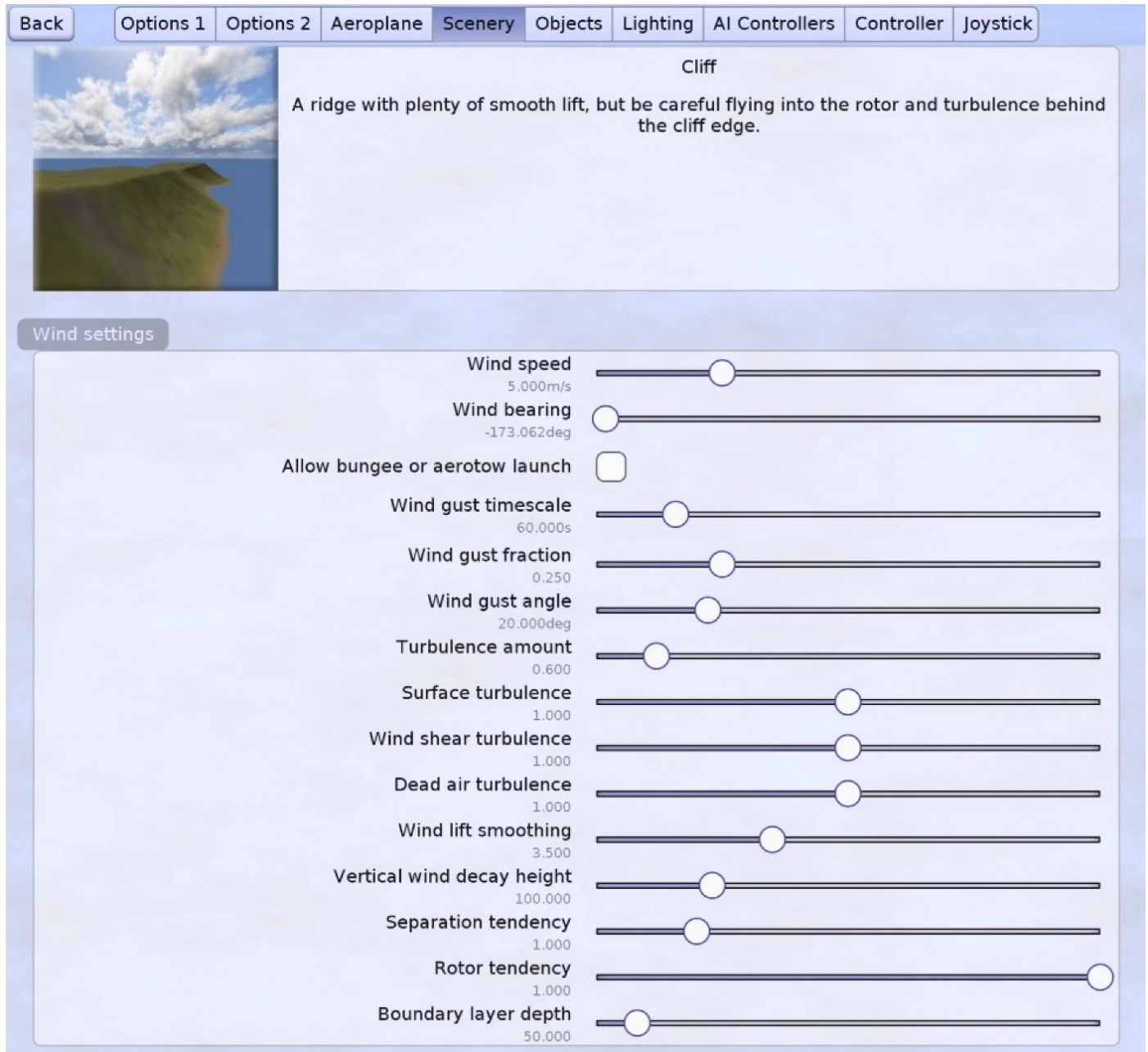
Figure 9: Flying site wind configuration settings.
