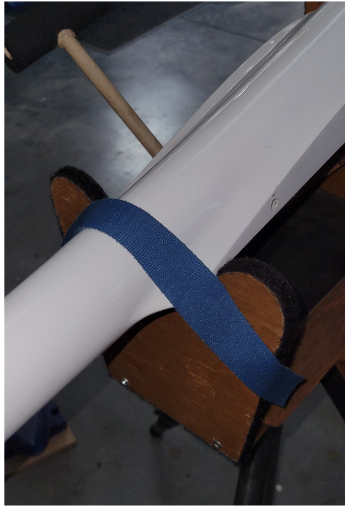
Photo 5 (left): The pan-heads let the side supports adjust and are tightened when you have it positioned where you want it. Photo 6 (right): All the stands have Velcro loop on the ends and use Velcro hook to secure the planes.
