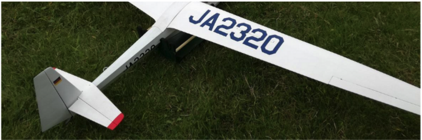
Photo 2: 1/5 scale ASK-18 by which I tested the ArduPilot Auto Soaring function.
