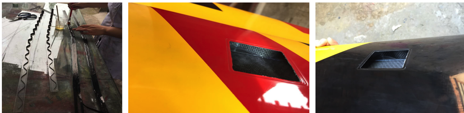
Photos 14, 15 and 16: The ASWS under construction and installed in the completed airframe. (images: Dr. James Hammond)
