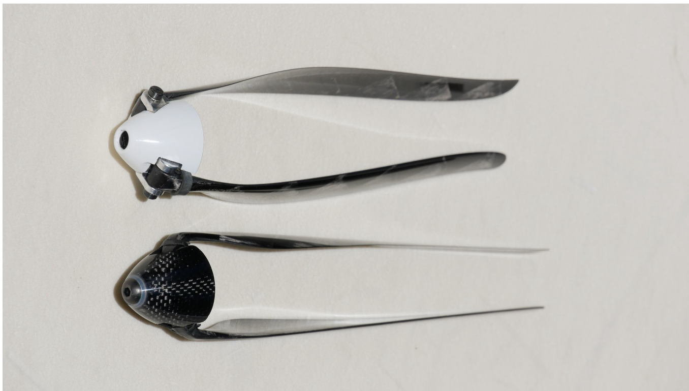
Photo 19: GM competition line 16x10 folding prop at the bottom, compared to the standard GM propeller of the same size.
