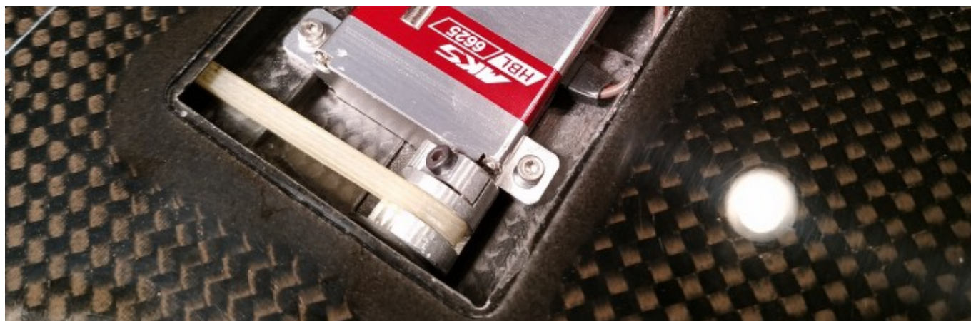
Photo 22: The excellent MP jet LDS system is provided with nice carbon servo frames for wing installation.
