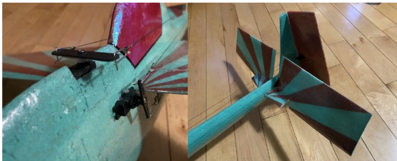
Pull-pull servo configuration and the resulting extreme deflections of the tail surfaces.
