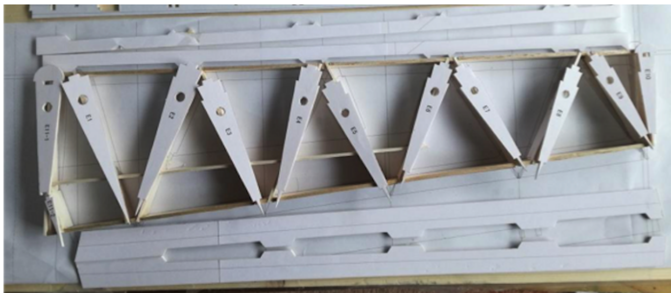
Photo 22: Elevator components placed on its assembly jig.
