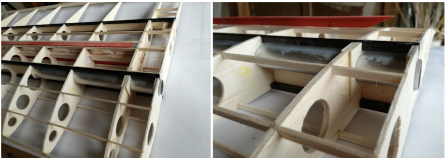
Photo 13: Center wing rib assembly after gluing is completed.
