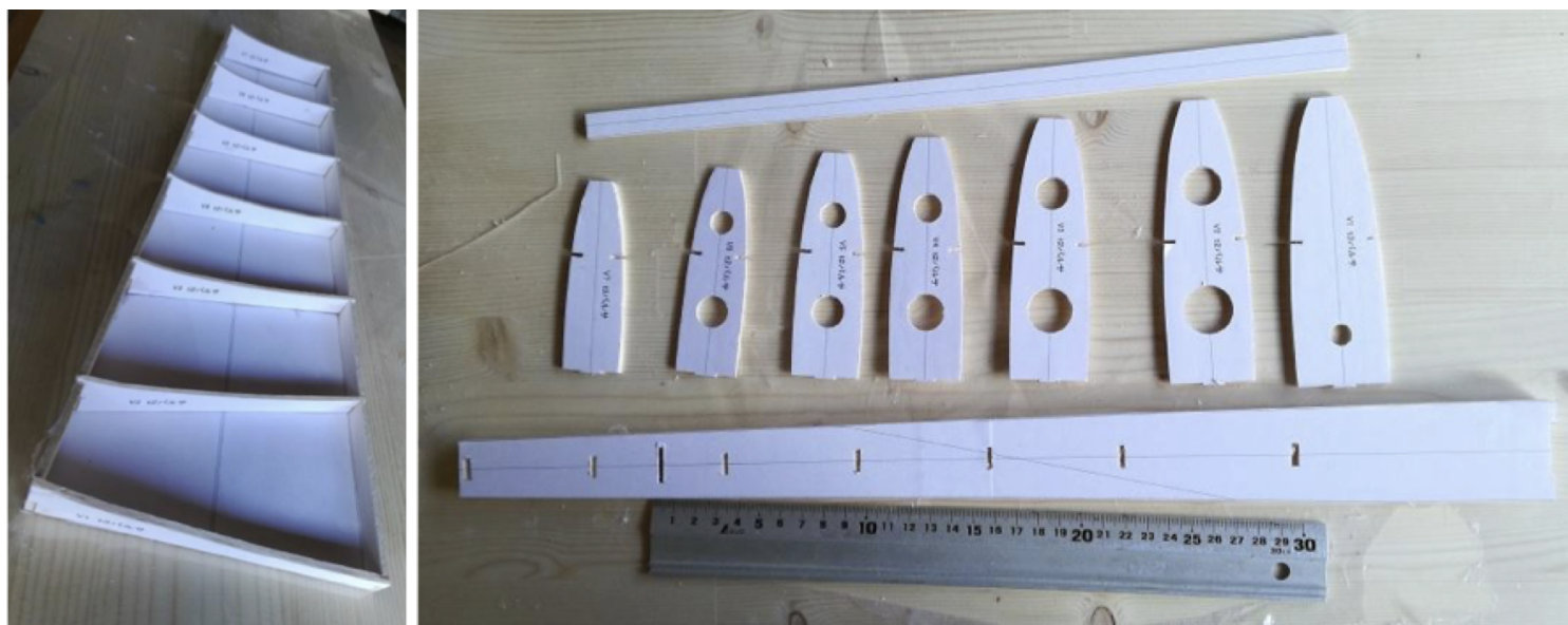
Photo 19: Assembly jig and parts of the vertical fin.
