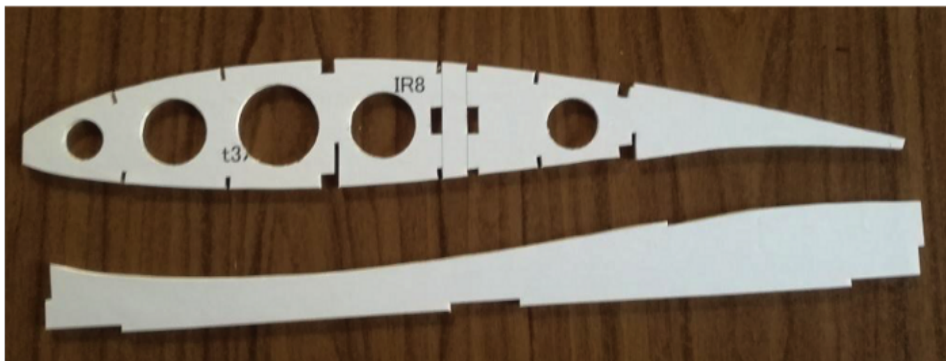
Image 8: Cut-out rib and assembly jig component
