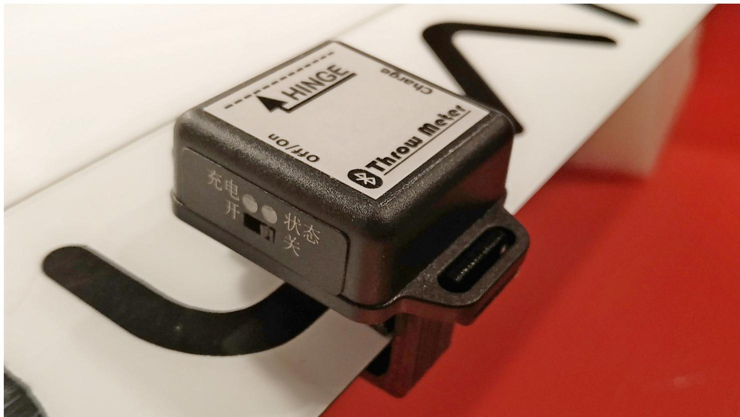
**Photo 1:** The RC Throwmeter mounted on the wing.
