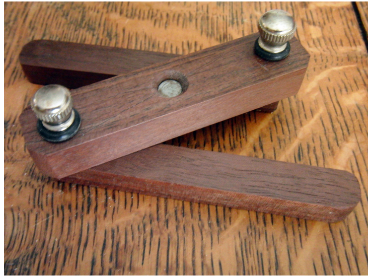
Photos 3 and 4: The basic parts, and the assembled center finder.
