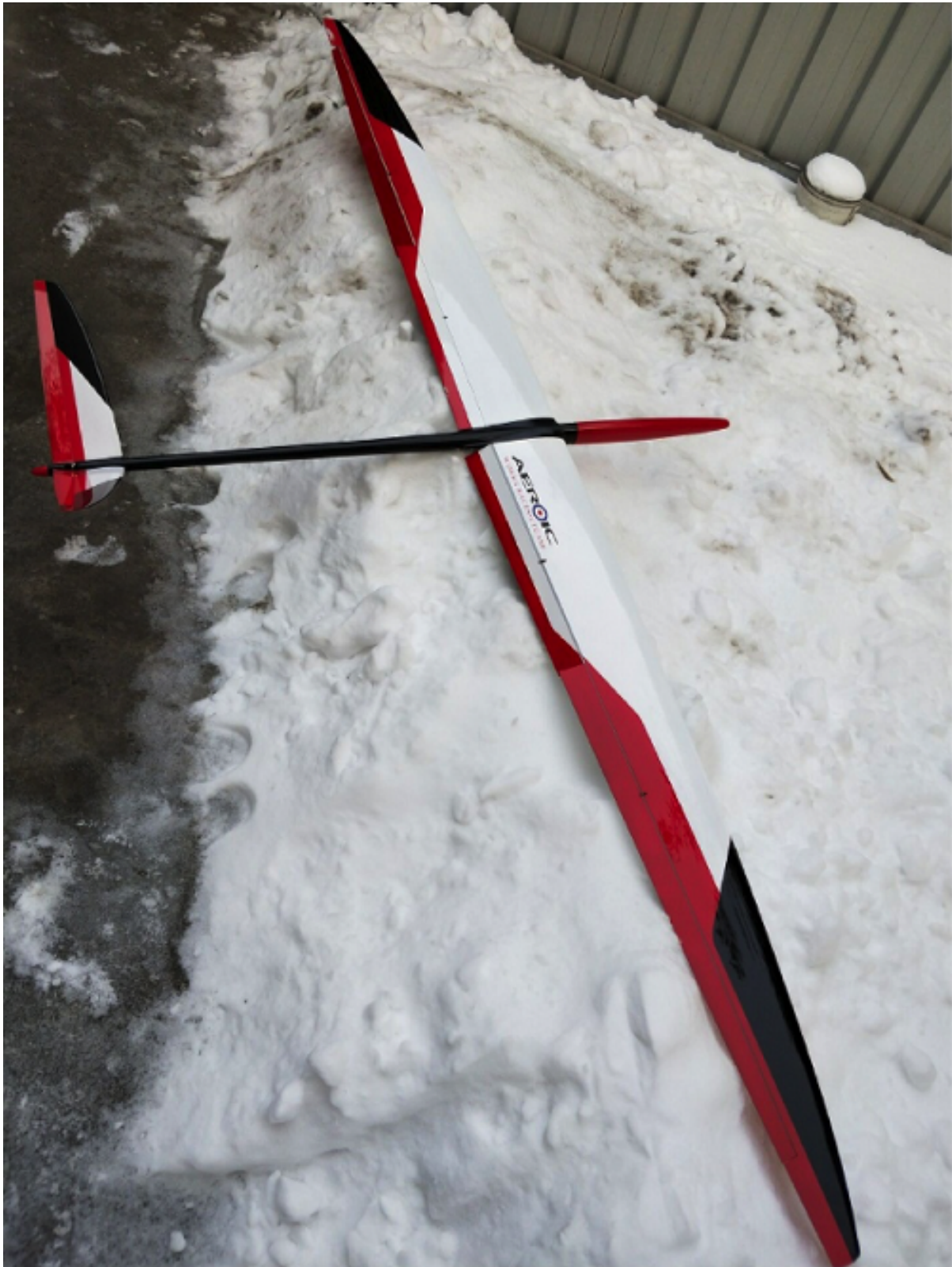
This shot shows the Redshift's 19:1+ aspect ratio — pretty high for a racer. (image: Julia Liu)
