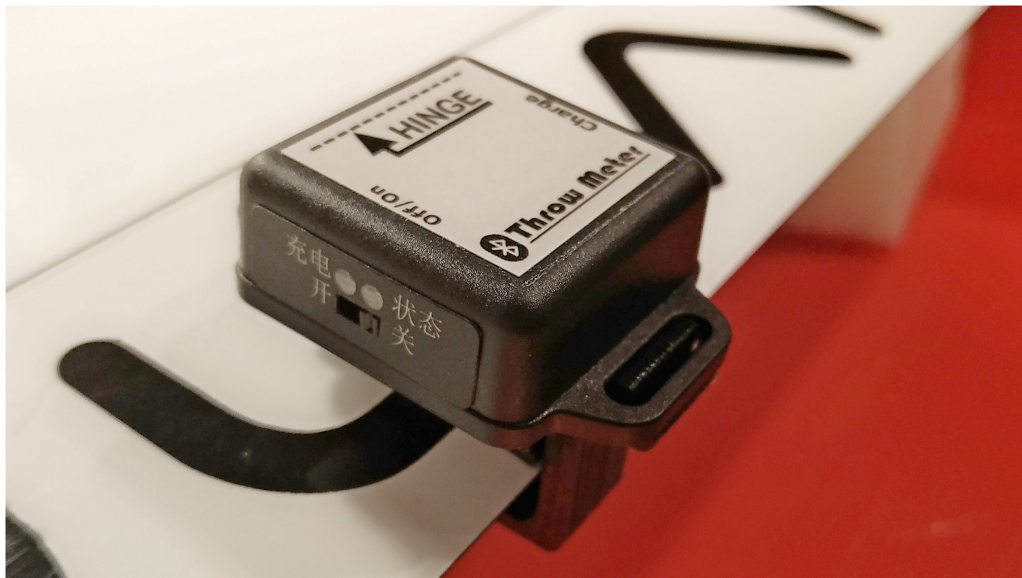
Photo 1: The RC Throwmeter mounted on the wing.
