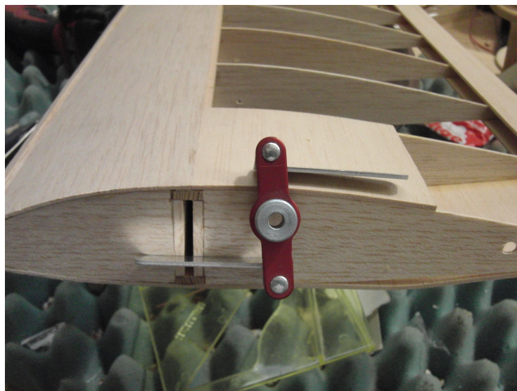
Photos 1 and 2: The Robart Hinge Point Drill Jig which I simply refer to as their center finder because that's what it actually does.
