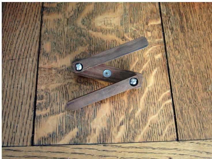
Photos 7 and 8: The finished center finder both with the marking pin on the left and, alternatively, a pencil on the right.
