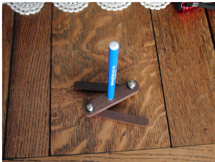
Photos 7 and 8: The finished center finder both with the marking pin on the left and, alternatively, a pencil on the right.
