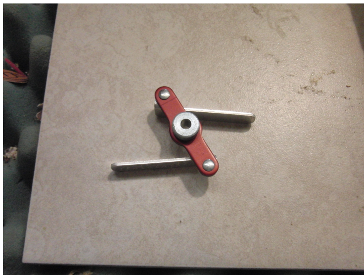
Photos 1 and 2: The Robart Hinge Point Drill Jig which I simply refer to as their center finder because that's what it actually does.
