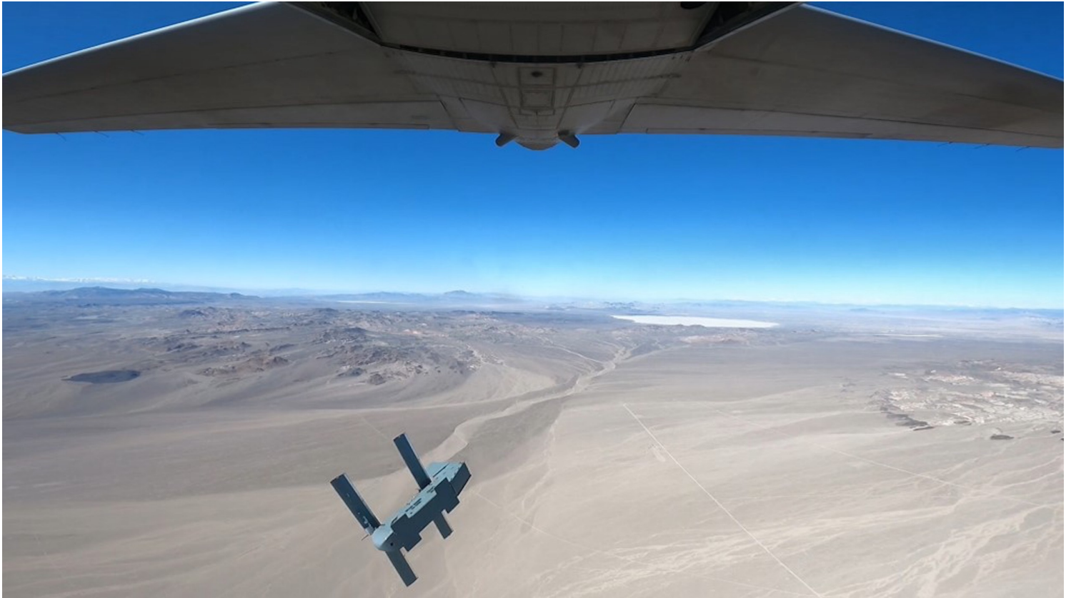
The view aft from the host C-130 'Hercules' as the Silent Arrow starts on its glide to the target.
