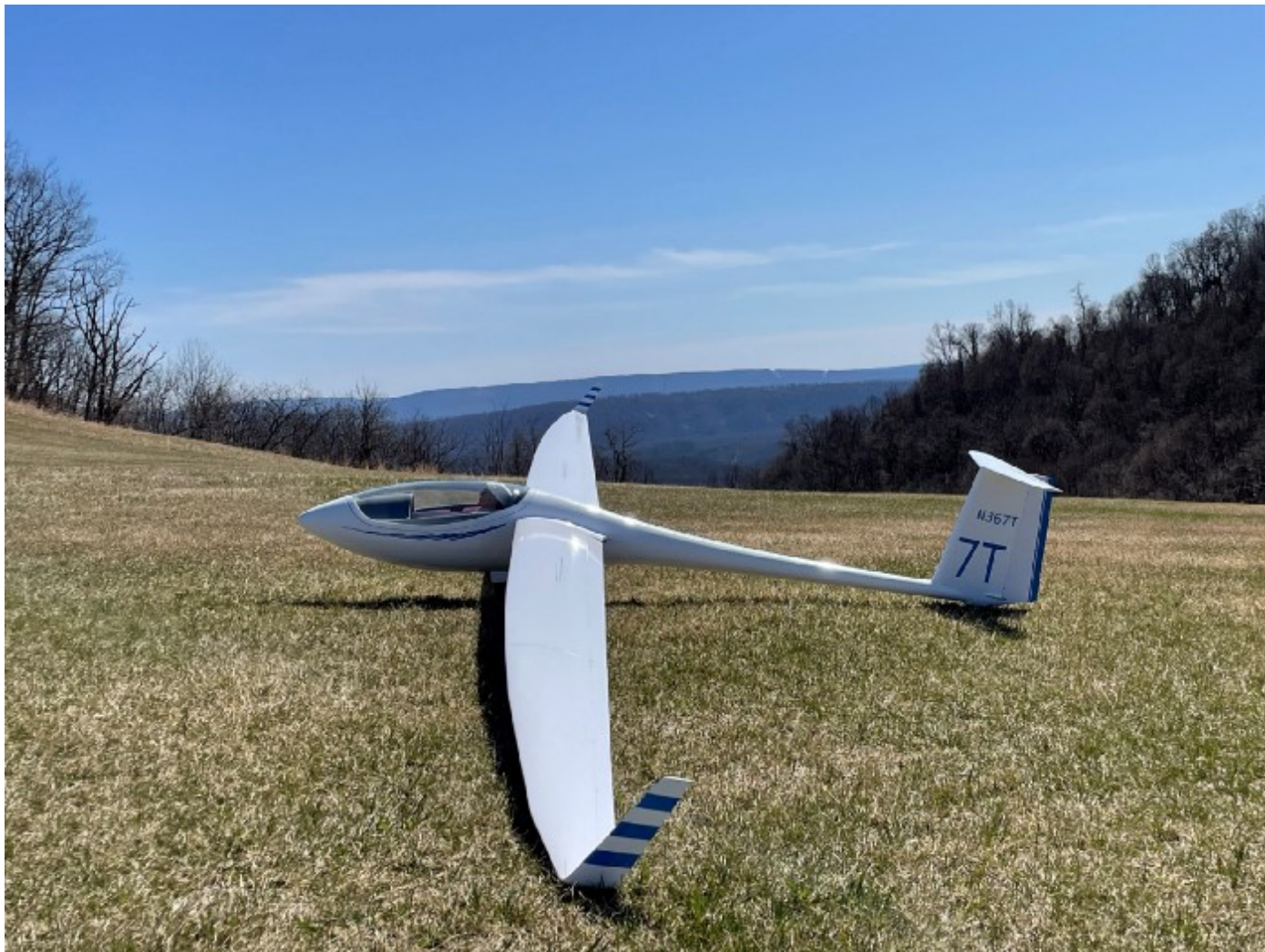
Photo 7: First flight for my winter project, a 6m ASG29. Powered with Rimfire 1.2 (Kv 450), 6S 5000mA and RFM 16x10 mounted with a Torcman FES system
