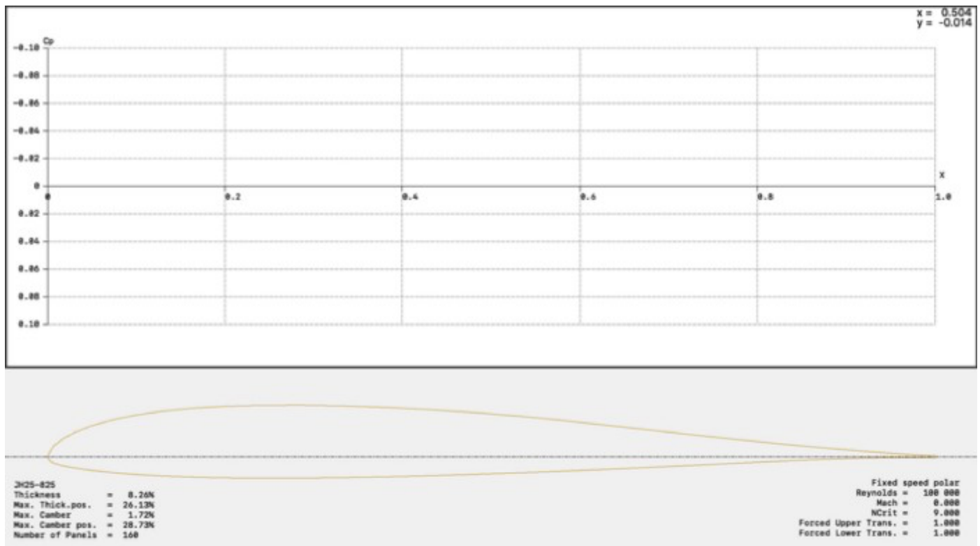
Figure 4: Profile of JH25 — an open source 8.25% thick section specifically designed for better control response.
